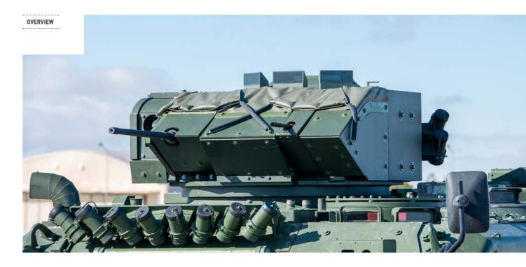
The SABER is a medium calibre oneman, power operated turret that can be fitted on wheeled and tracked armoured vehicles.
